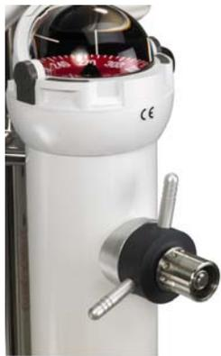
Position the wheel and engage it pressing with fingers on the flange. Fully engage the wheel while still pressing on the flange, and then release it. Turn the wheel slowly. The mechanism will engage automatically when turning the wheel.
