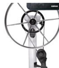
A Steer'n Go wheel can adapt : the customer just has to remove the notched belt and fasten it again to the Steer'n Go wheel.
