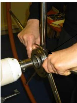
Position the wheel pressing with fingers on the flange.
