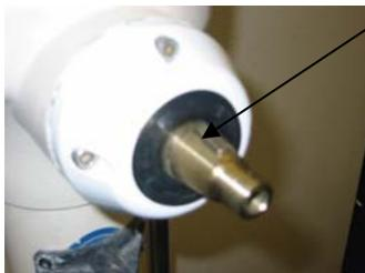
The drive shaft has a square key which will be needed when mounting the new Steer'n Go wheel.
