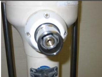
Put the nut and tighten it with the ratchet spinner.
