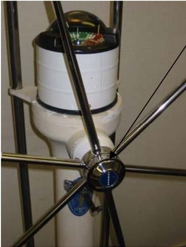
Put off the front friction brake.
